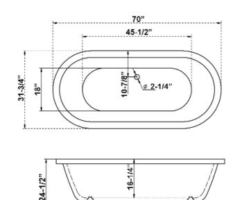
Overflow can be drilled. With overflow drilled this tub requires drain **5599E**. **Tubs that have been**
